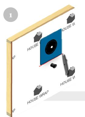
Using the Quickflash® panel as a guide, mark the length of the panel plus 1/4" on each side 2" above penetration onto the WRB and using a utility knife, cut a slit along the mark.
